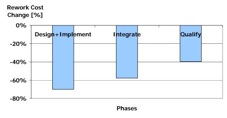
Figure 18: Rework cost comparison (TPCA pilot project)
